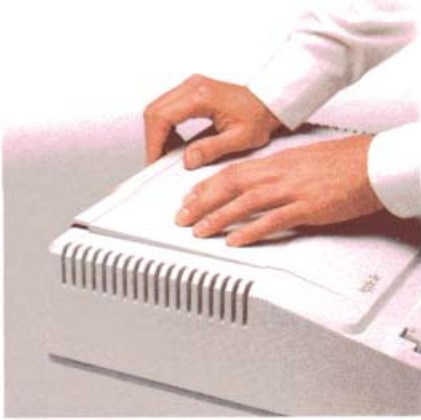
Figure 1-12 Replacing the Apple IIe top
