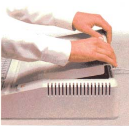
Figure 1-4 Removing the Apple IIe top
