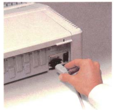
Figure 1-3 Plugging in the power cord
