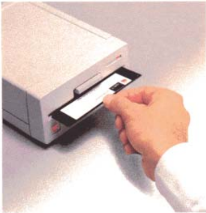
Figure 3-5 Inserting a 5.25-inch disk into a drive
