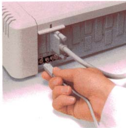
Figure 1-13 Plugging the monitor cable into the computer
