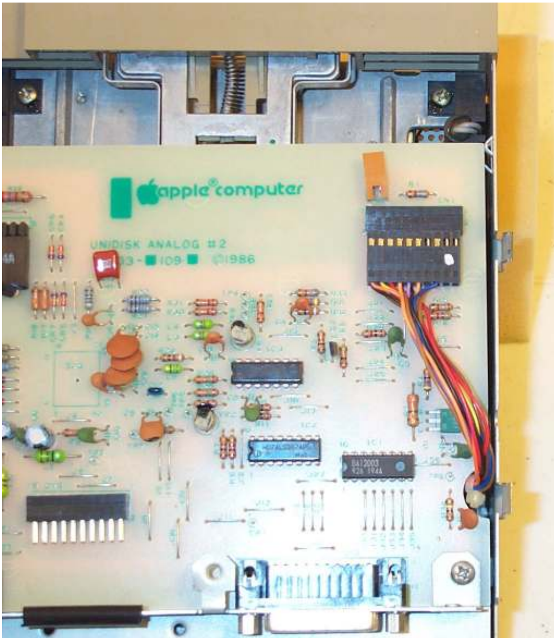
Figure 8. Location of the connector on the drive mechanism circuit board.
