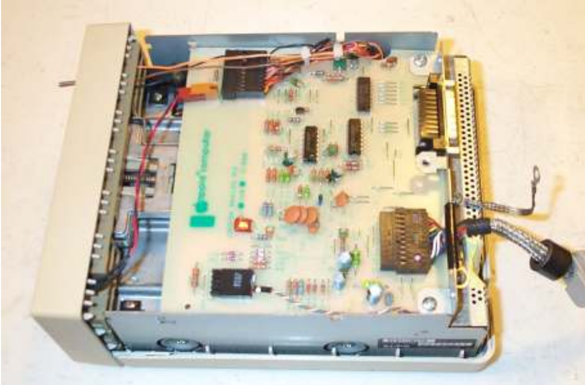
Figure 10. Electrical connections made, soldering done, electrical tape applied to solder connections, and wires harnessed.
