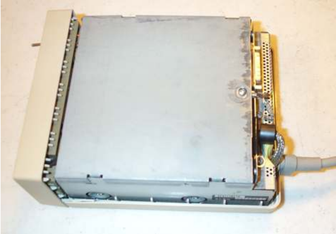
Figure 4. Case cover removed, looking down at the drive mechanism itself. Note that the metal lid is affixed by a single screw in the rear.
