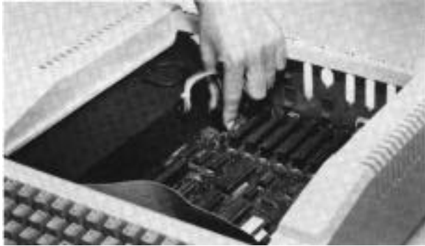
Plug Internal Cord Into Motherboard
