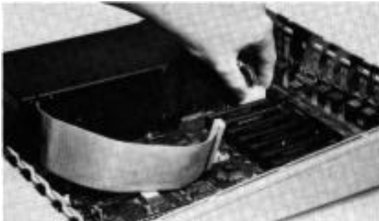
Plug Internal Cord Into Motherboard
