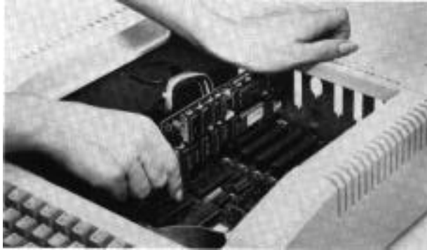
Insert Controller Card into Slot
