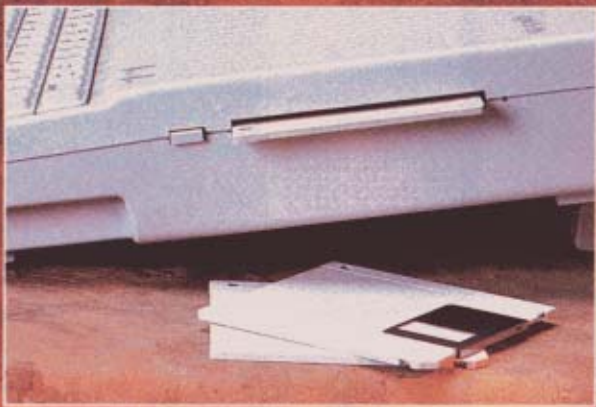
Figure 2: The internal 3.5-inch drive can store 800K of data.
