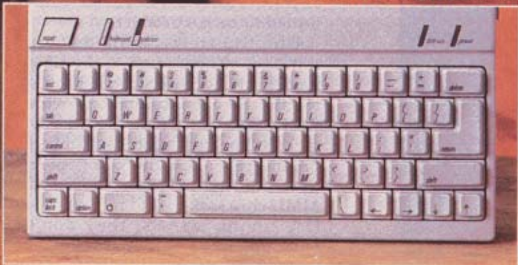
Figure 3: In addition to other slight modifications, the 80/40-column switch of the original IIc has been replaced by a sliding volume control.
