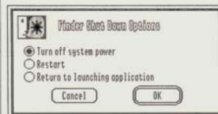
Figure 2: This Finder dialog box shows the options available when you select the Shut Down command.
