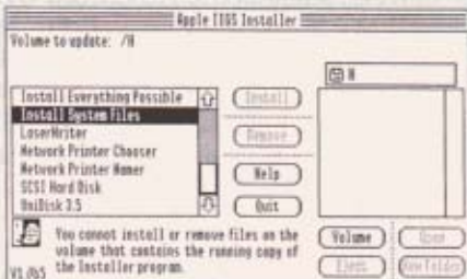
Figure 4: You can use Installer scripts to add operating-system files automatically to your standard boot disk.
