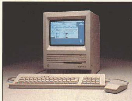
The Mac's Standard Keyboard, shown above, is also compatible with the GS, thanks to the ADB protocol. (Photo courtesy of Apple Computer.)
